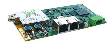
The Xeta9 Emancipator is an extremely capable, flexible, low cost industrial Frequency Hopping Spread Spectrum (FHSS) and Digital Transmission System (DTS) 900 MHz software defined radio (SDR). The module utilizes a XetaWave patent pending Dual Decode Digital Architecture™ that offers superior receiver performance.
